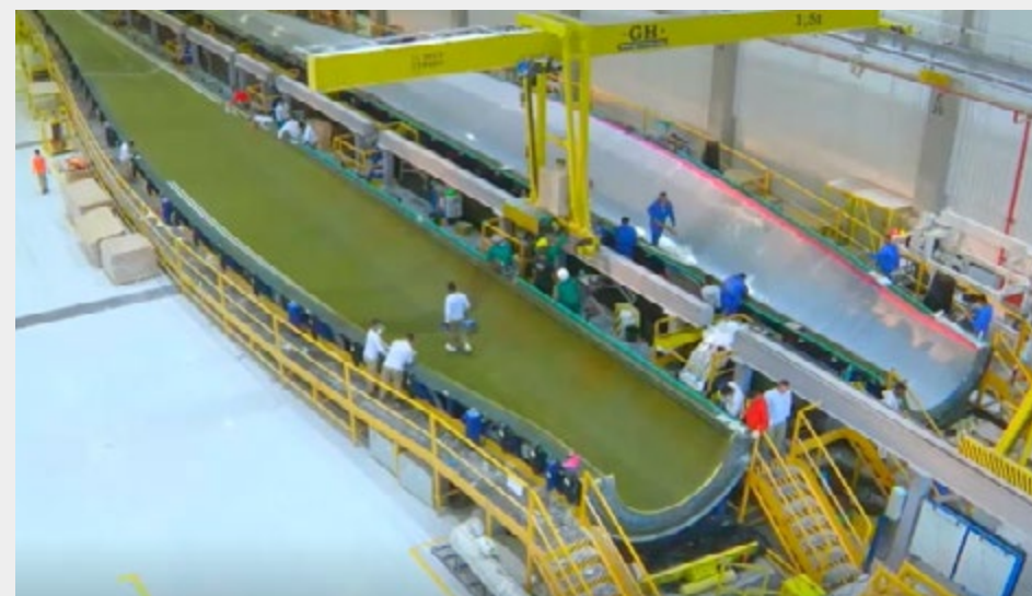
1 Preparation and cleaning of the mold and laying of several layers of fiberglass (inner layers).
