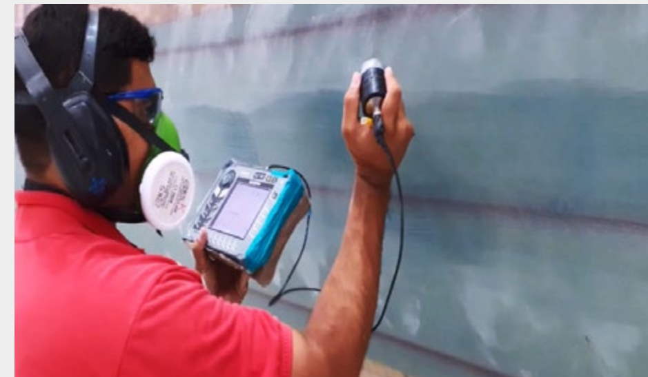
7 The blades go from the molds directly through quality inspection, which includes the use of ultrasound technology. Particularly, all bindings are evaluated.
