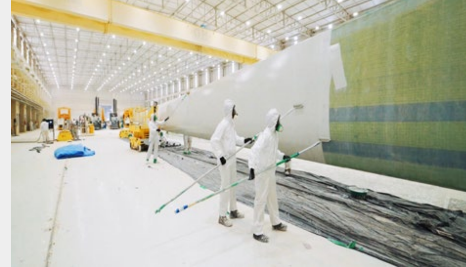
8 Finally, the blade is painted, balanced, and after final assembly is completed, packed.
