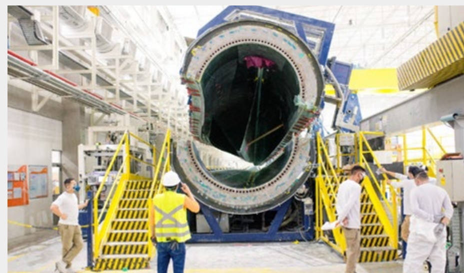
5 The spar flange and web are inserted and glued, so that one shell is separate from the other.
