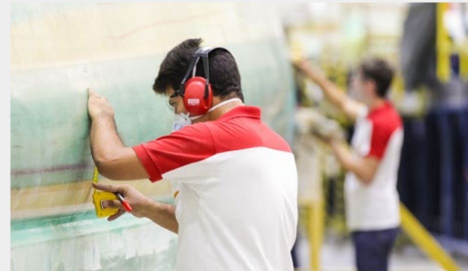
3 The insertion of further layers of fiberglass (on the outer surface area).
