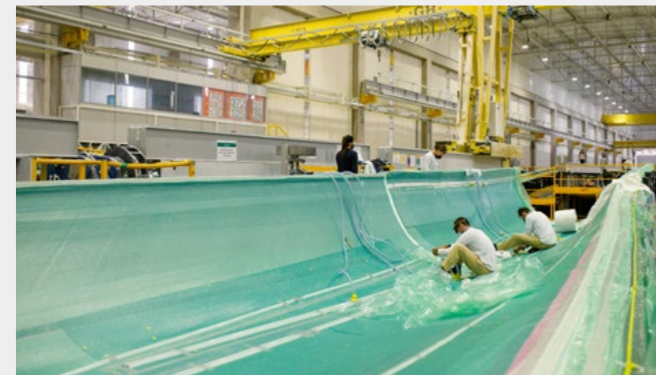
4 A vacuum bag is produced with the infusion of epoxy resin that goes through a chemical process for hardening called curing.
